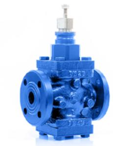
In order to avoid seat & plug wearing issues we recommend not to exceed 2 bar (2FGBB) & 8 bar (2FSA) & 12 bar (2FAAB) differential pressure.
