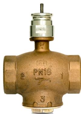
**2TBB.T** Series 2-way valves, bronze body, with threaded connections up to 2", brass plug, stainless steel stem. Temperature applications -10 °C to 150 °C (Please check on our data sheet DBL521e pressure rating for fluid temperature higher than 120°C).
