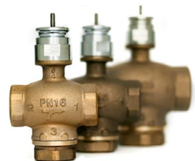
**3TBB.T** Series 3-way valves, mixing or diverting, bronze valve bodies with threaded connections, brass plug, stainless steel stem.
